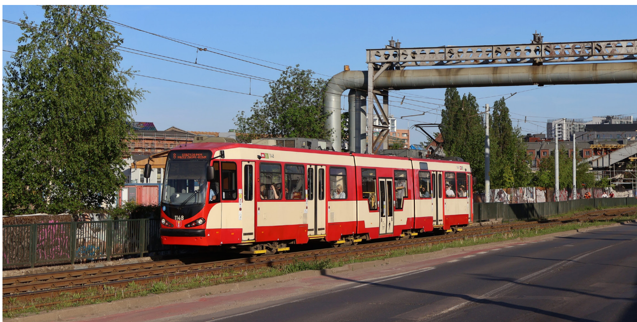
Partially low-floor Duewag N8C-MF 01 tram in Gdańsk equipped with ENIKA electrical equipment.
