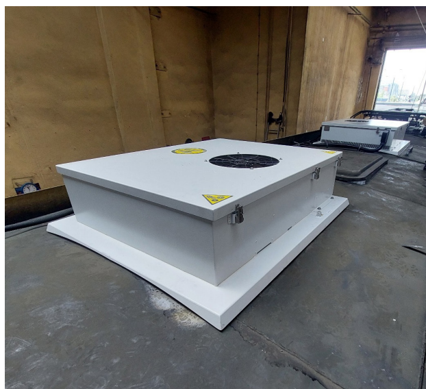
Example of an iGORRA air conditioning system installation on a Protram 204WrAs tram.
