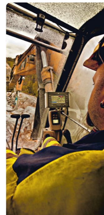
The graphic display of ExcaDrill is user-friendly. The angle and depth measuring system is included. ExcaDrill can be also equipped with a video monitoring camera. This allows the remote visual control of the drilling process on graphic display.
