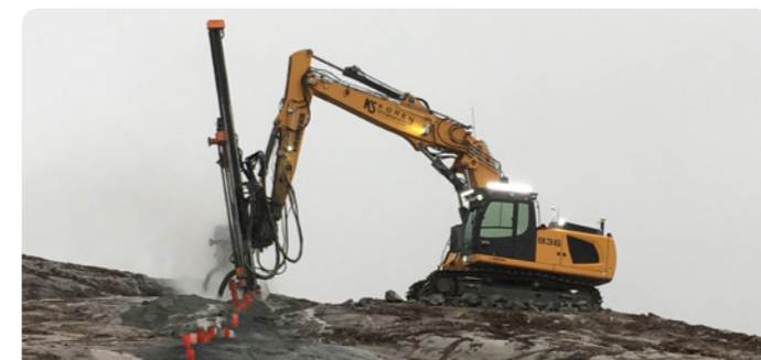
The graphic display of ExcaDrill is user-friendly. The angle and depth measuring system is included. ExcaDrill can be also equipped with a video monitoring camera. This allows the remote visual control of the drilling process on graphic display.
