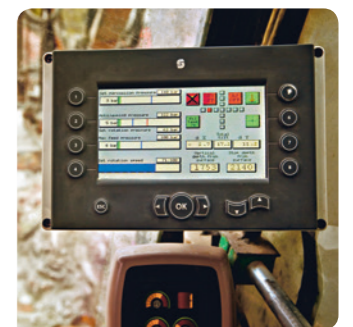
The graphic display of ExcaDrill is user-friendly. The angle and depth measuring system is included. ExcaDrill can be also equipped with a video monitoring camera. This allows the remote visual control of the drilling process on graphic display.
