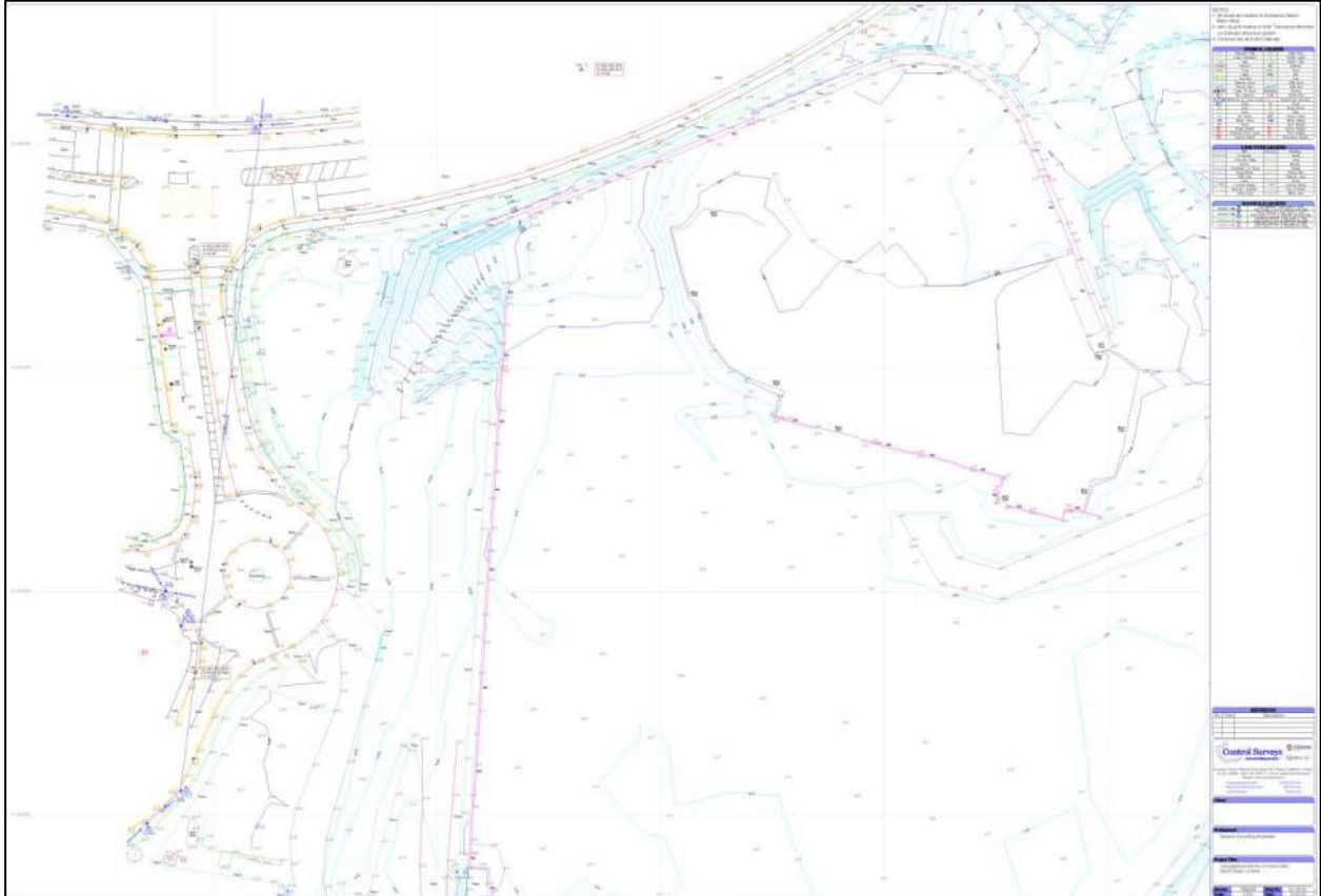
Figure 1-1: Image showing existing site topography of northern side of the site
