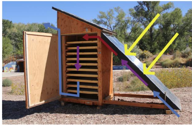
Figure 5 Indirect Solar Dehydrator (McCann, 2022)
