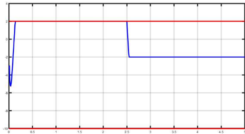
Figure 11.55: The second state ( x_2 , in blue) as a function of simulation time. It obeys its constraints (red) throughout the simulation.
