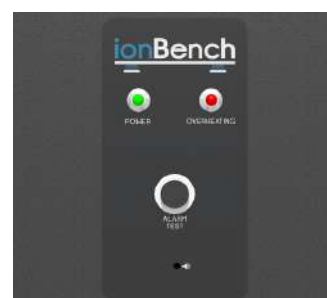
Overheating temperature alarm
