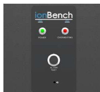
Overheating temperature alarm
