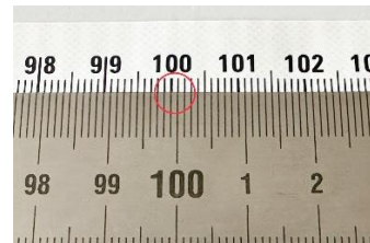
Figure 65 1m on the reference scale is 1mm longer than on the tape measure
