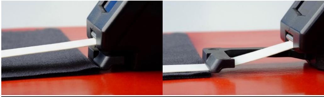
Figure 42 Measuring failure because of large distance between objects and measuring tape outlet
