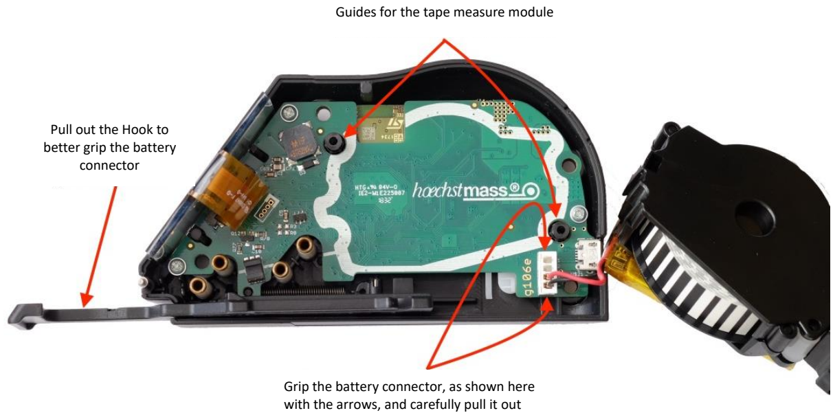
Figure 53 Remove measuring tape module
