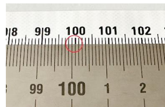
Figure 67 1m on the reference scale is 1mm shorter than on the tape measure
