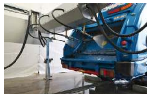
Shower Hopper cleaning the inlet
