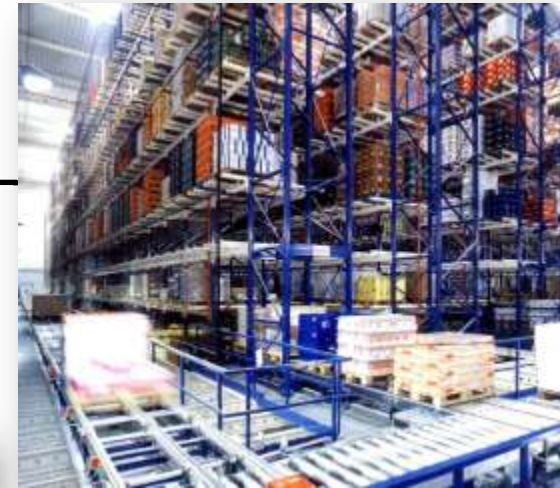
Putaway Pallets to ASRS HBW
