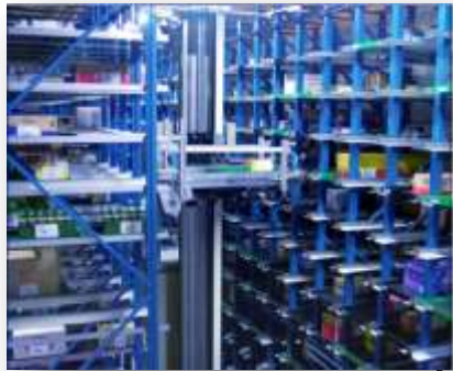
Mini-load automatically extracts and selects trays
