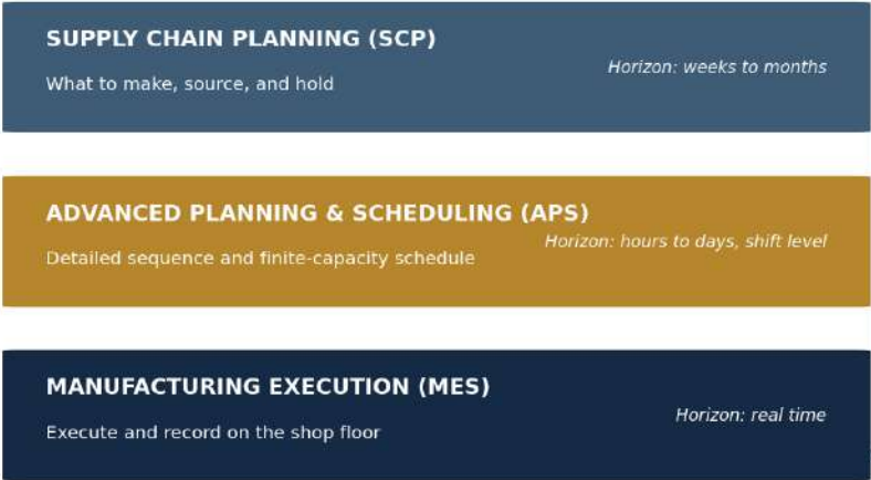
Figure 3. The manufacturing planning stack. APS is the detailed-scheduling layer between supply planning and shop-floor execution, and conflating it with either is the most common buyer error.
