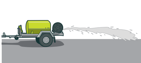
FIGURE 9: Examples of using water to dampen dust at unsealed worksites
