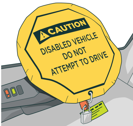
FIGURE 17: Example of mobile plant that cannot be used until it has been fixed
