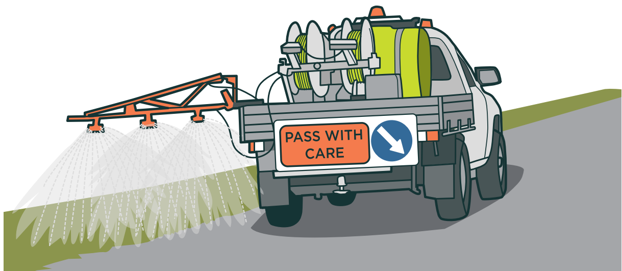
FIGURE 11: Example of automated spraying system to limit worker exposure to the chemical being used (also keeps worker in a safer location inside the vehicle)
