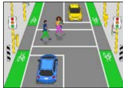
Dedicated signalled pedestrian crossings (Not intersection)
