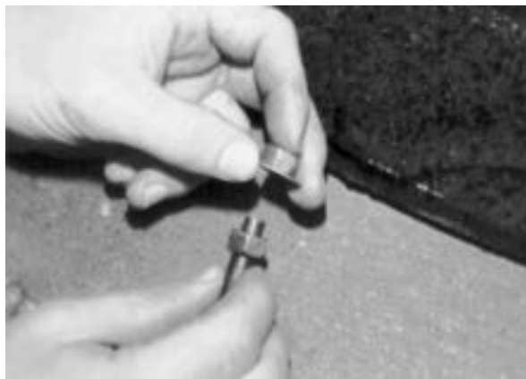
Placing two nuts and a washer onto the stud
