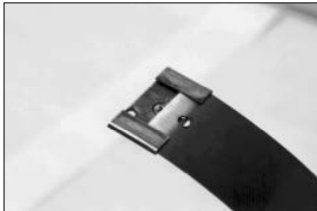
Sliding the ring stabilizer onto the ring
