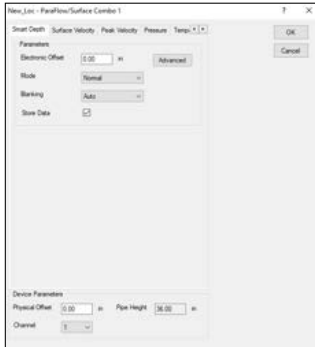
Edit ParaFlow/Surface Combo 1 Parameters dialog (Smart Depth tab)
