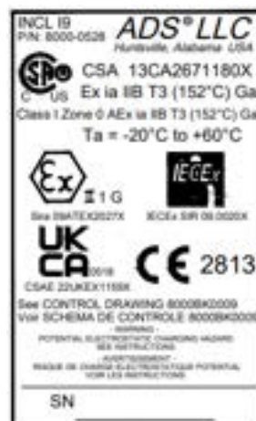
Long Range Depth (CS6) ATEX, IECEx, CSA, UKCA Certification Label
