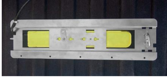
Attach ParaDepth/ParaFlow Sensor to Sensor Bracket
