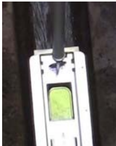
Position the Hook Through the Loop on the Sensor Bracket
