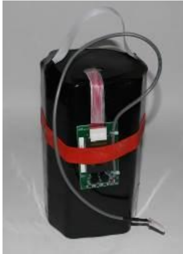
12-volt battery pack with PCB
