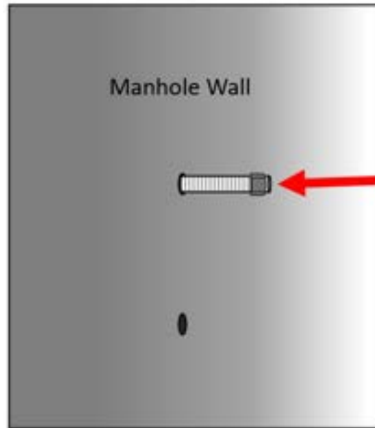
Installing the First Anchor Bolt
