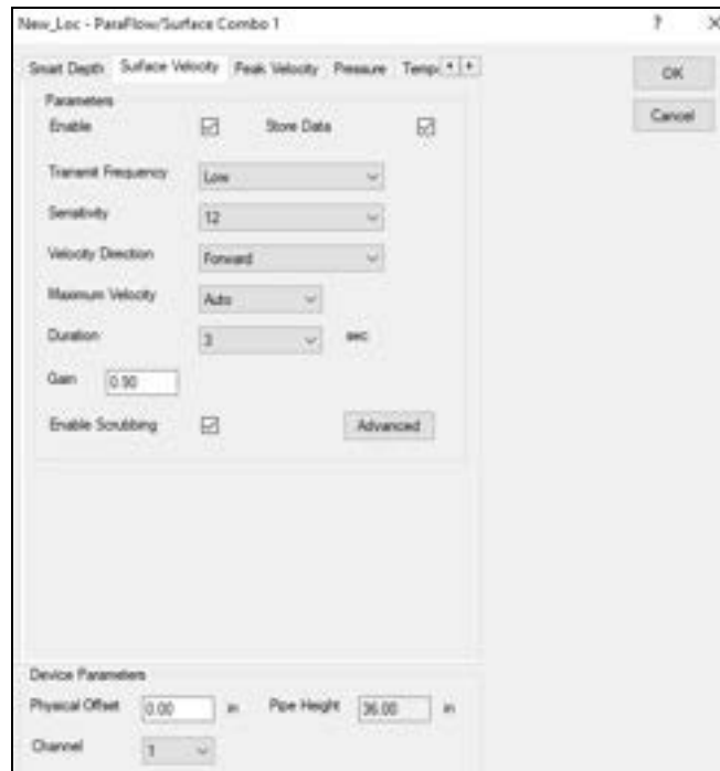
[location name] – ParaFlow/Surface Combo dialog displaying Surface Velocity tab
