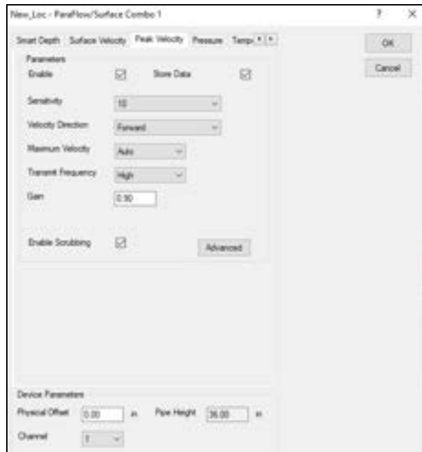
Edit ParaFlow/Surface Combo 1 Parameters dialog displaying the Peak Velocity tab
