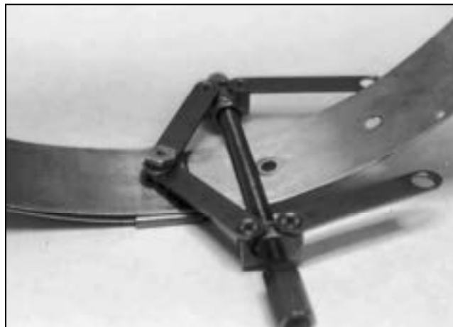
Attaching the spreader bars
