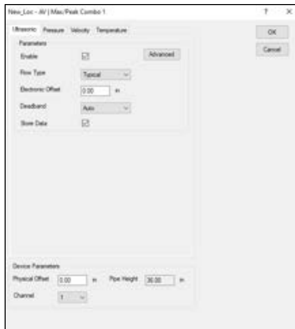
Edit the AV|Gated 1 parameters showing the Ultrasonic tab
