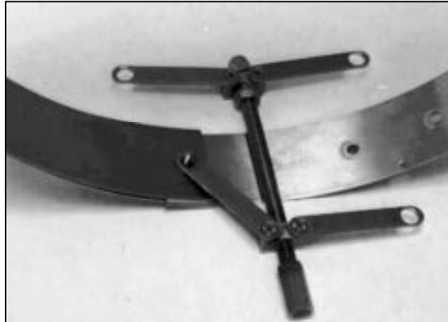
Orienting and attaching the spreader mechanism
