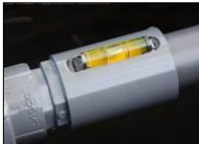
Ensuring Mounting Bar is level
