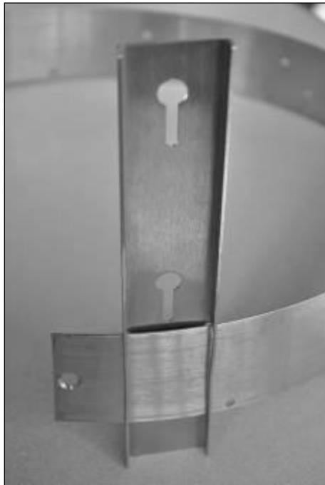
Sliding the Ultrasonic Depth Sensor mounting plate onto the ring, in the Surface Combo configuration
