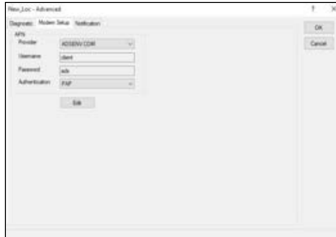
Advanced Device - Modem Setup dialog
