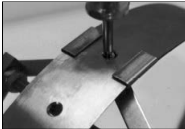
Tightening the spreader mechanism screw and hex nut
