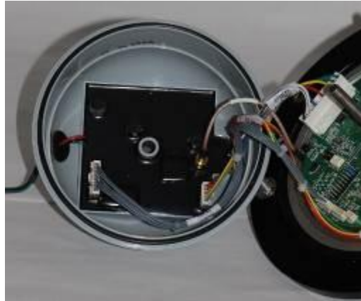
Power regulator dome with IS regulator board
