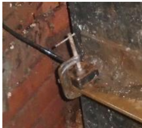
Inclinometer attached using a Stainless Steel Clamp
