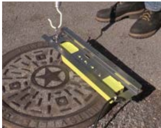
Sensor Bracket Securely Looped on Pole Hook
