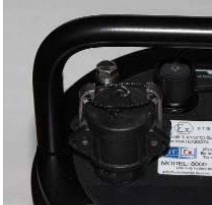
SIM card enclosure with plastic tie
