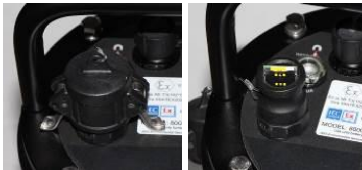
SIM card enclosure locks released (left) and enclosure cap removed (right)
