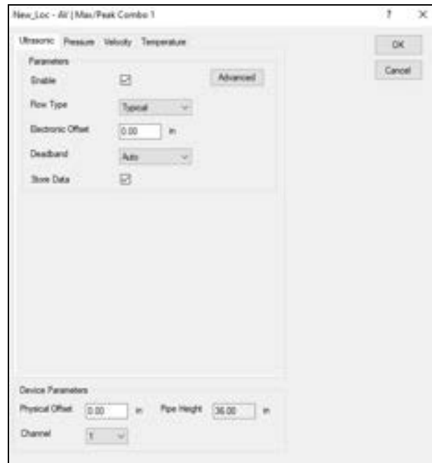
Edit AV|Max/Peak Combo 1 Parameters dialog showing the Ultrasonic tab
