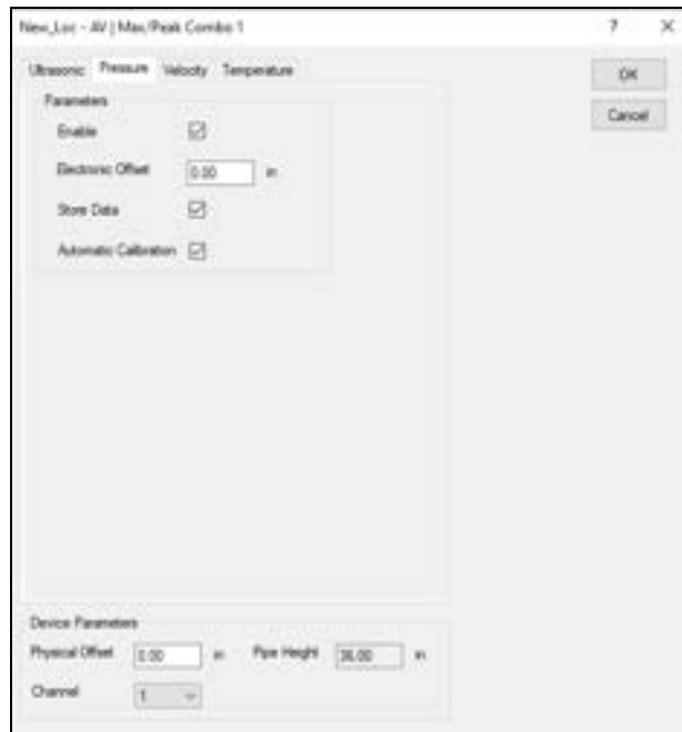
Edit AV|Max/Peak Combo 1 Parameters dialog displaying the Pressure tab
