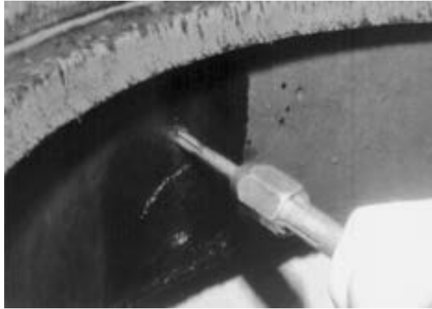
Using the tap to thread the hole
