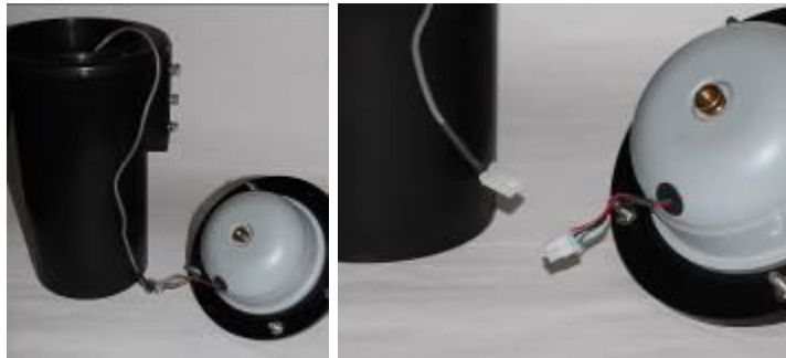
Placing the top next to the monitor (left) and disconnecting the cables at the plastic white connectors (right)
