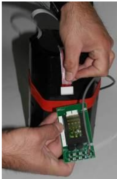
Disconnecting the PCB from the battery pack
