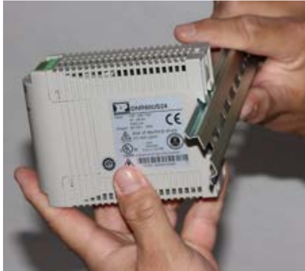
Sliding the top edge of the DIN rail into the wedge on the back of the power supply
