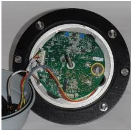
TRITON+ top with processor board attached
