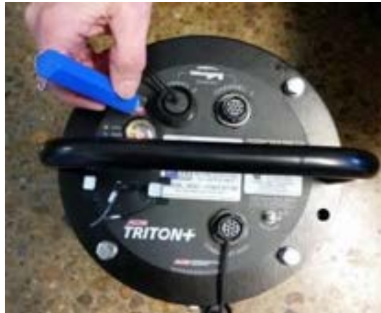
Codes Initiate after Removing Magnet from Contact with Monitor Top
