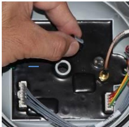
Blue fuse removed from the regulator board
