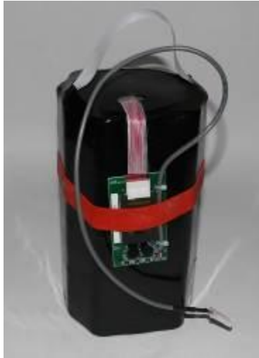
12-volt battery pack with PCB
