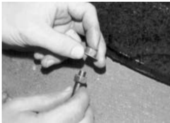
Placing two nuts and a washer onto the stud
