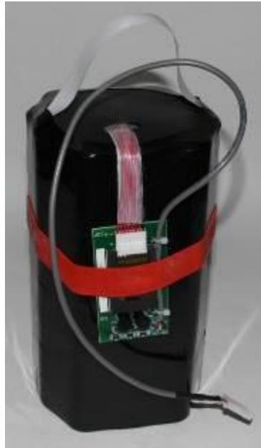
12-volt battery pack without retainer plug
