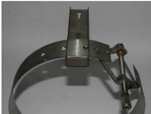
Properly attached spreader mechanism (with Ultrasonic Depth Sensor mounting plate on ring, configured for a Surface Combo)
