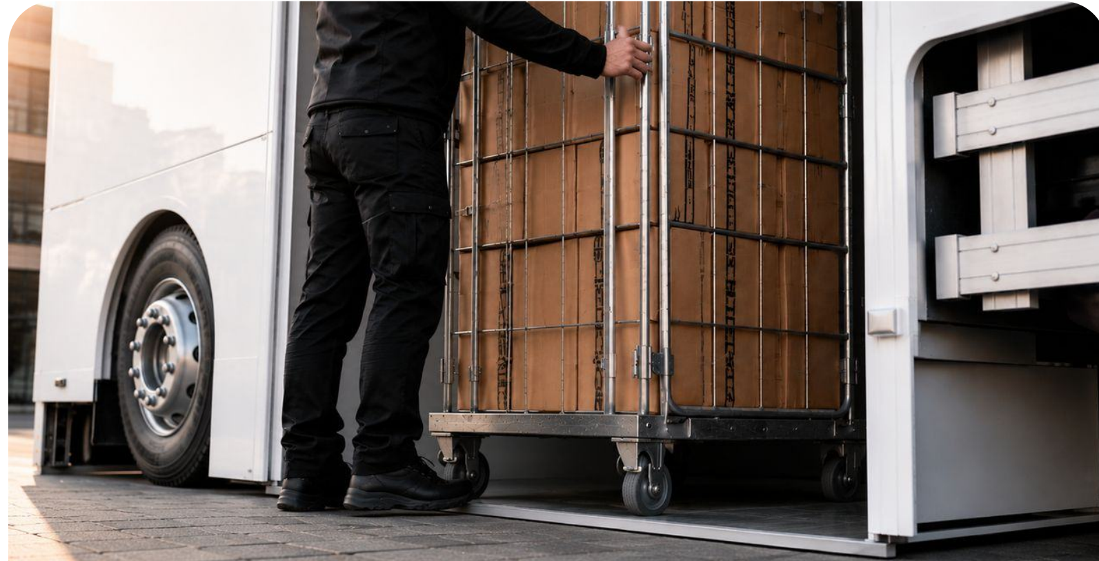
Internal lift with continuously variable height adjustment
