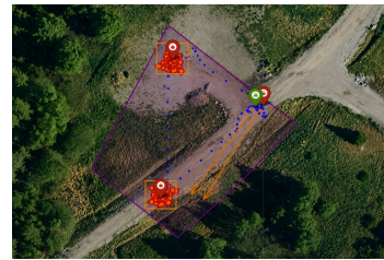
Fig. 3. Hotspot clustering. Blue: the drone's flight track. Orange: one fire seen in many frames, grouped into a single fire.
