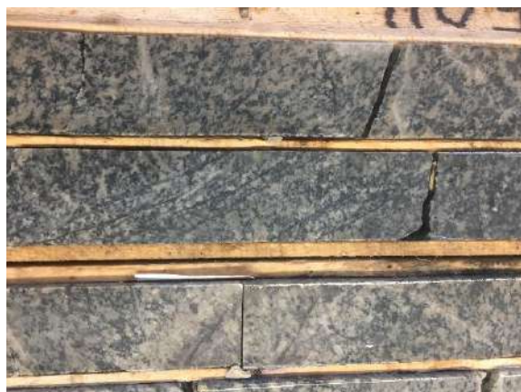
Plate 7. Neoproterozoic, medium-grained tonalite, Mag Zone, WL-17-29.
