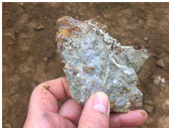
Plate 28. Pyrite-quartz stringers in altered porphyry, Red Ochre Complex.
