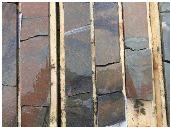
Plate 27. Altered feldspar porphyry with stringer pyrite, Red Ochre Complex.
