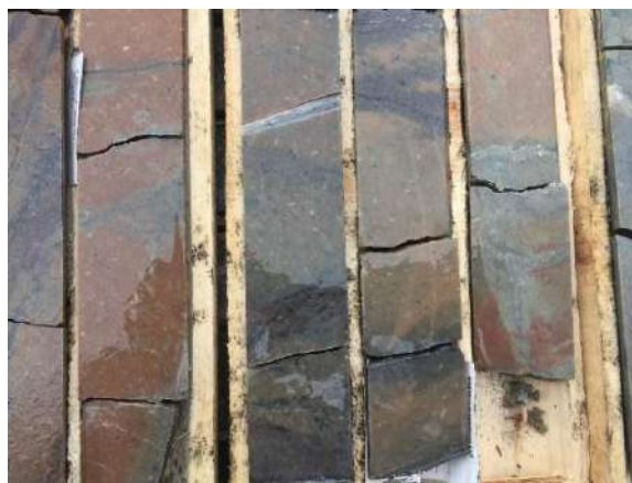
Plate 6. Reddish-brown feldspar porphyry, Red Ochre Complex.
