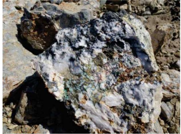
Plate 10. Quartz-tourmaline, chalcopyrite, hematite and malachite, Alder Zone.
