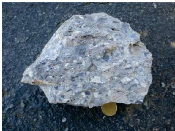
Plate 2. Typical clast-supported, purple polymictic Rogerson Lake Conglomerate.
