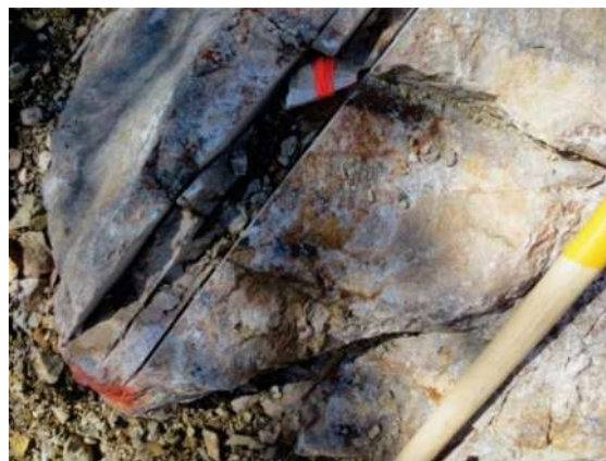
Plate 30. Flat quartz vein with pyrite, Birch Zone.
