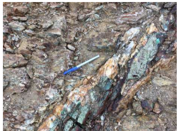
Plate 17. Chalcopyrite-rich V_2 vein, Elm Zone.
