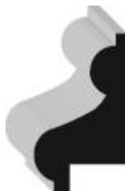
1 3/16 x 1 3/8 PANEL MOULD WITH 1/2" OFFSET
