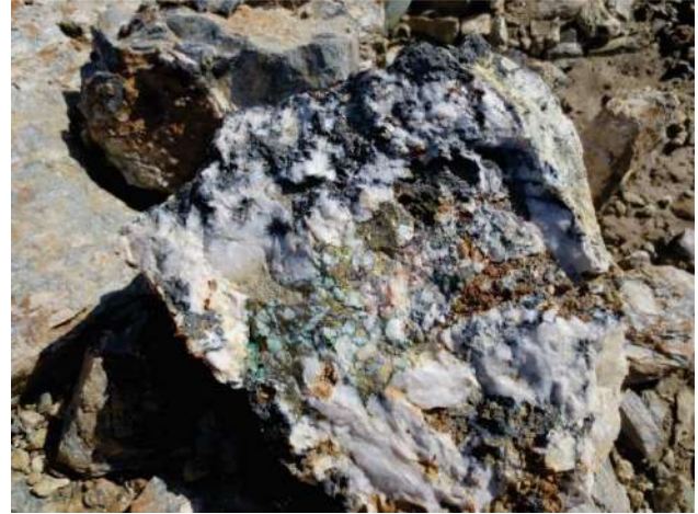
Plate 10. Quartz-tourmaline, chalcopyrite, hematite and malachite, Alder Zone.
