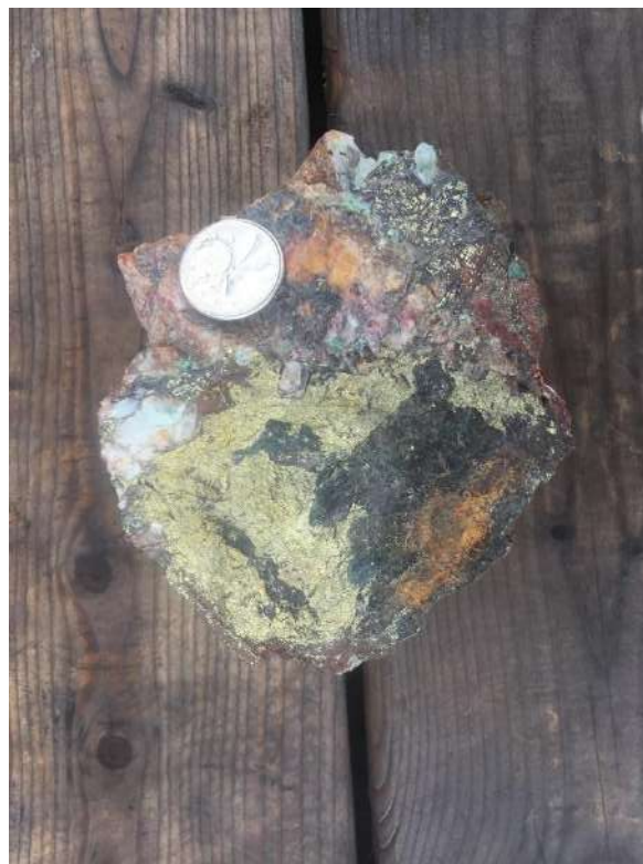
Plate 23. Raven Zone grab sample, with chalcopyrite in quartz, assayed 273.8 g/t Au.
