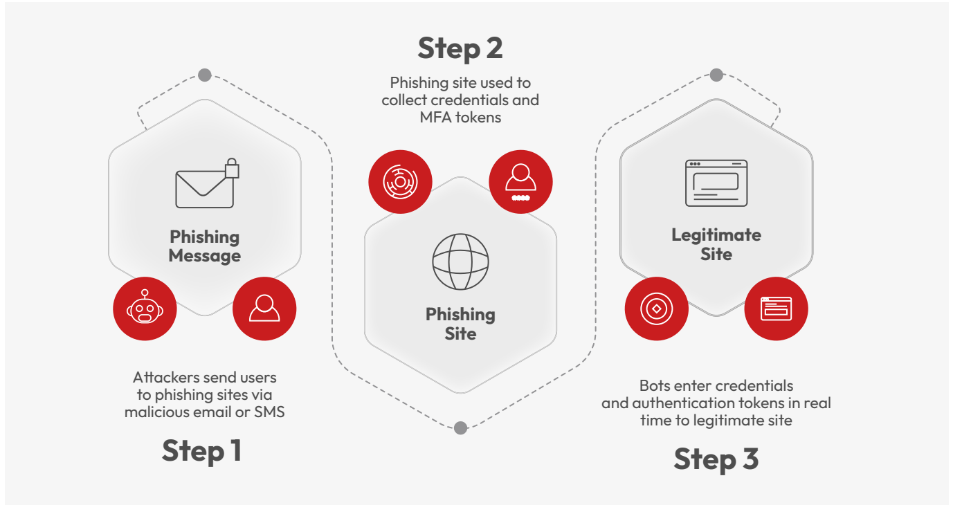
Figure 1: How Phishing Reverse Proxy Works
