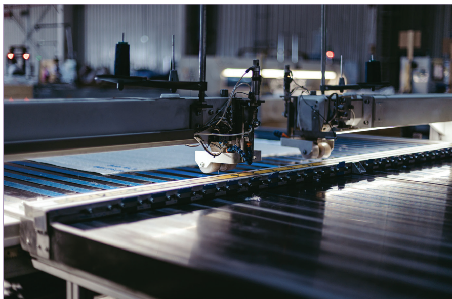
Fig. 2: The assembly of multi-layer sub-segments of the wind blade lay-up can be made with those production lines in a highly accurate and efficient manner © InCom Group
