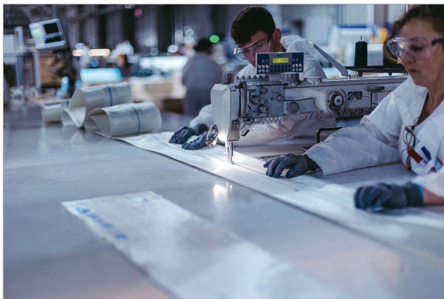
Fig. 1: Stitched fibreglass preform for a wind blade © InCom Group
