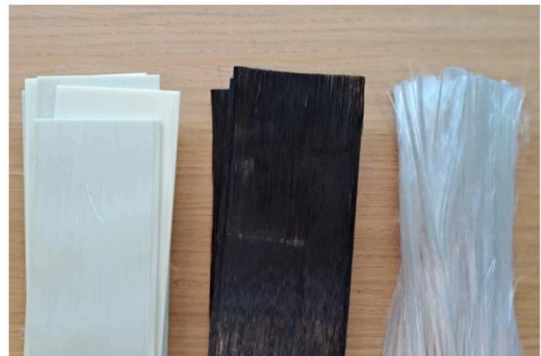
Owens Corning epoxy-based composite material used to produce wind turbine blades (left), after thermolysis treatment (center) and after calcination (right). Source | Composite Recycling
