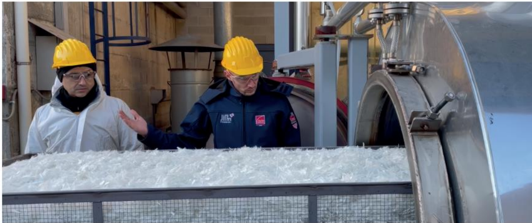
Through pyrolysis, organic parts (thermoset resin) and inorganic parts (glass fibres and fillers) are separated enabling components to be recycled independently in a closed loop approach.
