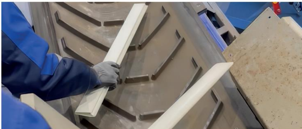
The closed loop glass recycling process begins with finished thermoset composite materials, which are seen here being fed into the line at the beginning of the process.
