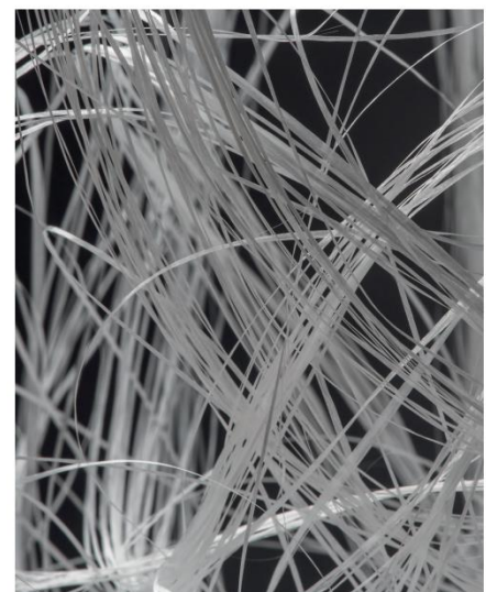
Manufactured from a combination of post-industrial circular glass fibres and traditional glass input materials, SUSTAINA Loop maintains the same high level of performance and quality as virgin glass fibre.
