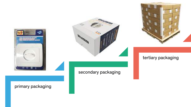
Figure 3: Examples of different types of packaging used in the installation sector.
