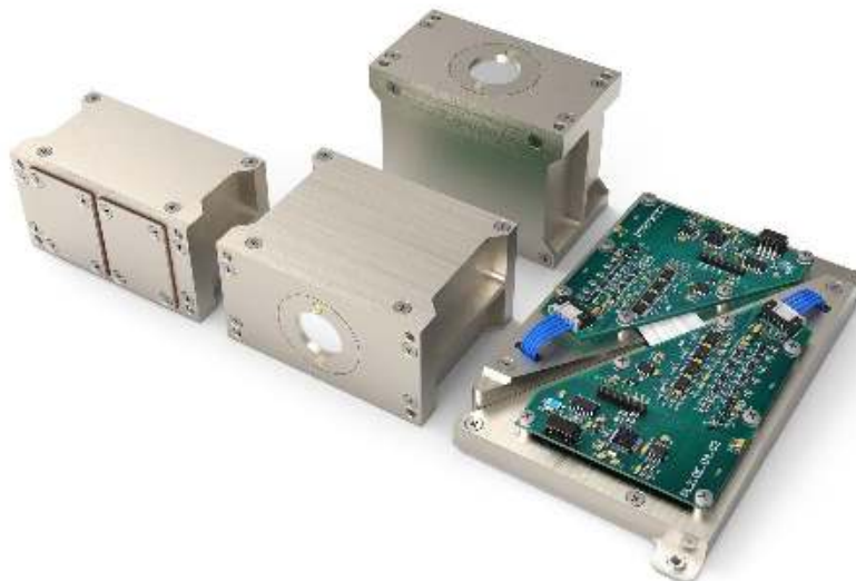
Figure 5 – The Complete Magnetospheric Monitoring Suit consists of minimum 4 units and covers all energy ranges from plasma to relativistic.
