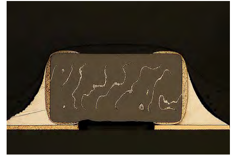
Capacitor tin plating height detection
