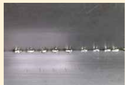
Corner spot welding thickness 0,6 mm
