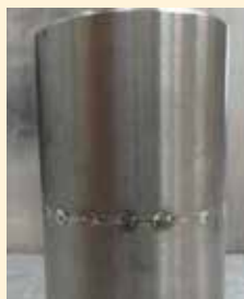
Pipe butt weld Ø 31.75 x 2 mm
