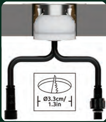
Connect the led ground light with other led ground lights
