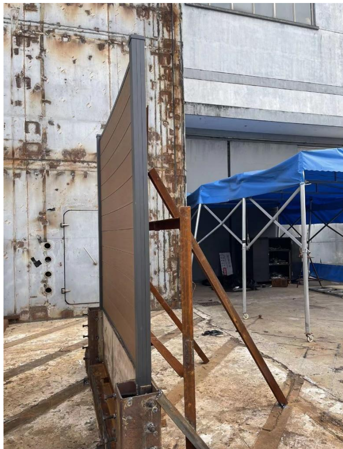
Photo No.3 After Wind load Testing
