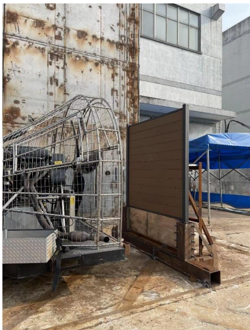
Photo No.1 Before Wind load Testing
