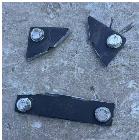
Photo 5. The fence specimen was damaged by the wind load at wind speed of 100 mph
