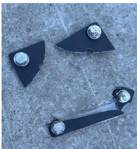
Photo 6. The fence specimen was damaged by the wind load at wind speed of 100 mph
