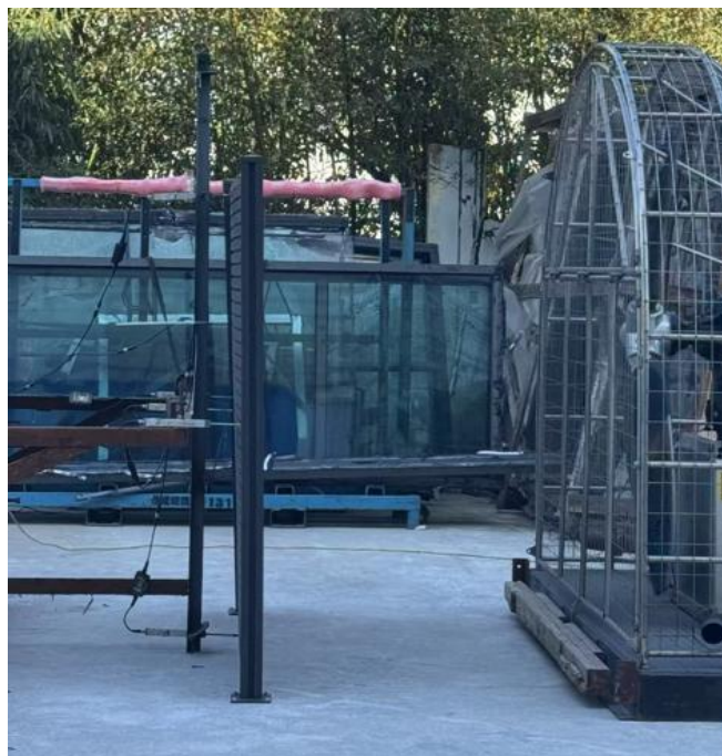
Photo No.2 The specimen was under wind speed loading test
