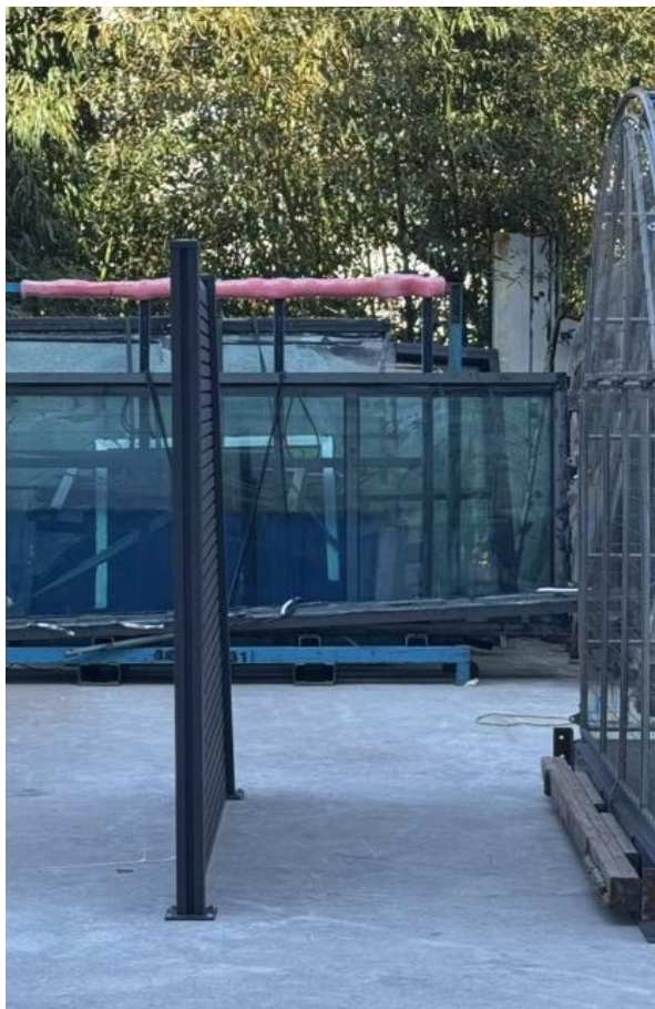
Photo No.3 The fence specimen after a wind speed of 90 mph testing
