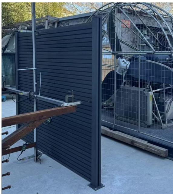
Photo No.1 The specimen was set on cement ground with transducers before wind load testing
