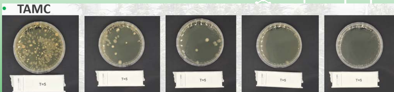
Figure 2: TAMC measurement at Brightlabs on day 5 ranging from 10^{-1} to 10^{-5} .
