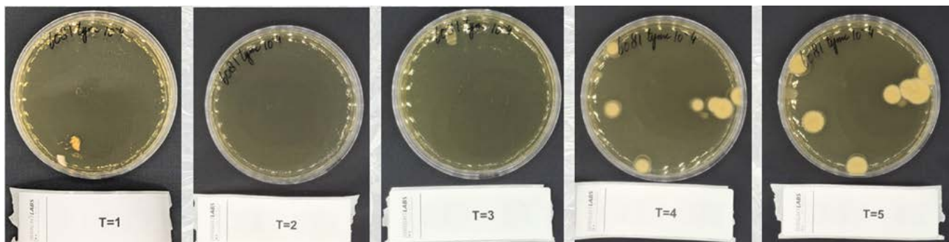
Figure 1: TYMC measurement at Brightlabs, day 1 to 5, dilution 10^{-4}
