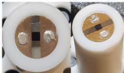
Front and perspective view of an ALTP. The side length of the central sensor element is ca. 1 mm, while the outer column measures ca. 8 mm across.
