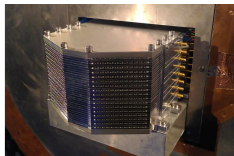
Antenna prototype stacked from 33 modules, compactly forming two 2D antenna arrays. Beams are steered perpendicularly to the modules by feeding them different signals.
