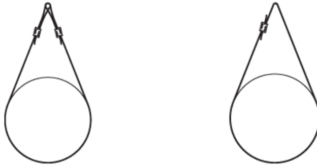
FIGURE 2—HANGING METHOD – SINGLE POINT SADDLE CONFIGURATION
