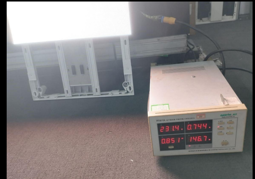
MP-480V2@ common cathode tech , 500*500mm cabinet size , 8S, 5300nit, 146.7W
