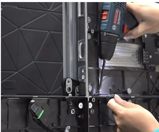
Lock between Cabinets with the Hex Socket Head Screws M6*6.
