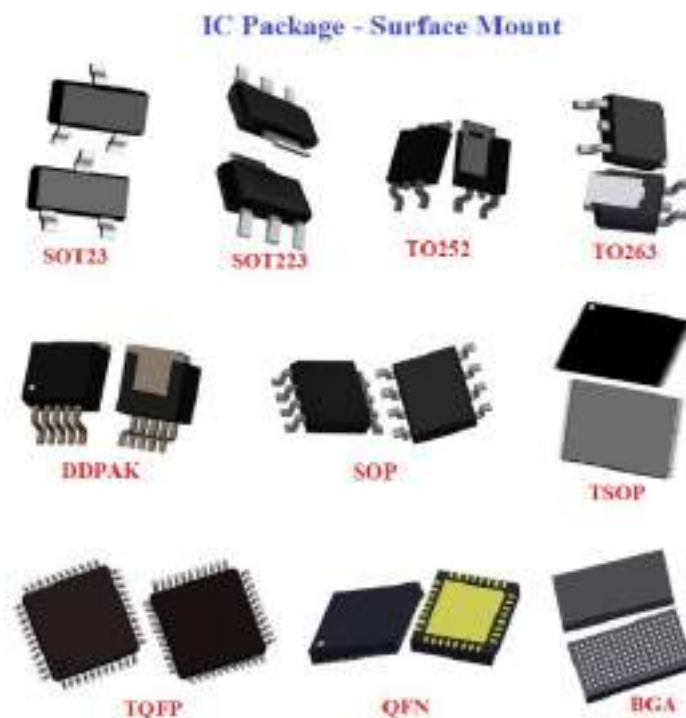
Fig 3. IC Package-Surface Mount
