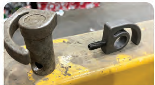
Steel-wire twister component compared with PlasLOC+ twister component.
