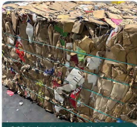
OCC bale with uniform PlasLOC+ spacing visible.
