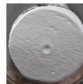
Fig. 3. Al-base contact-layer with a top-layer of Ag on a 3,000 mm² Al Milliken-conductor
