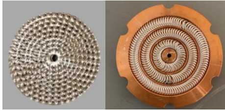
Fig. 5. Flex-elements. Embossed Ag-plate (Flex1, left), and a canted coil spring flex-element (Flex2, right)
