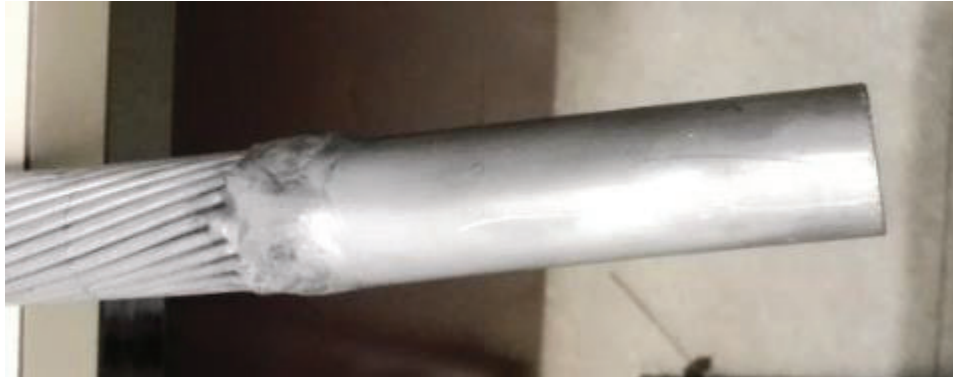
Figure 2-6: Weld of a solid rod at the end of a stranded cable
