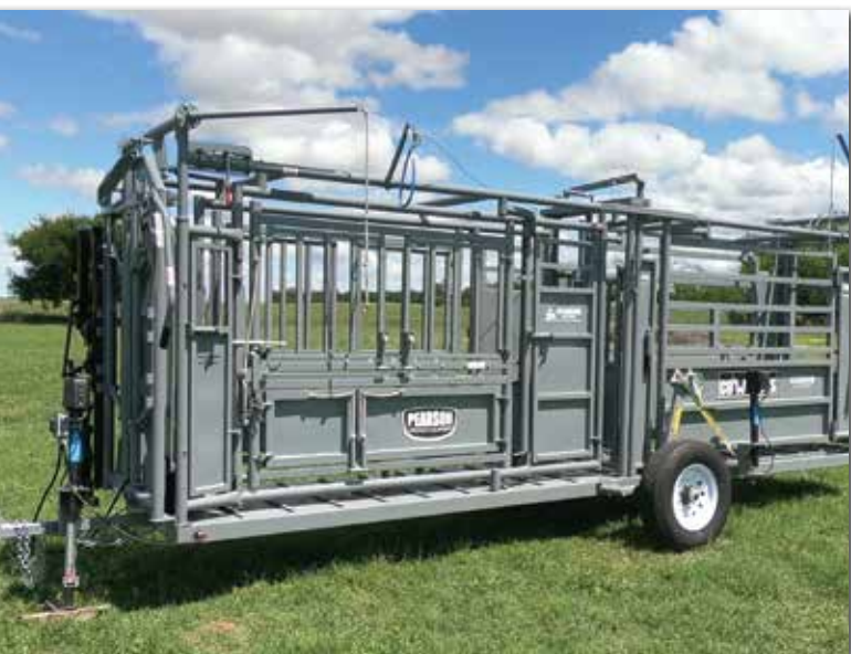
Portable System Designed to Work Cattle On the Go
