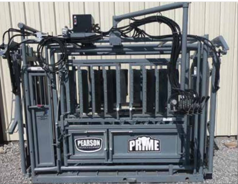
Drop Arm Controls and Neck Viewing Window
