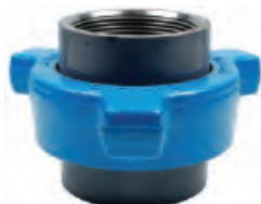
Figure 206 Threaded 2000 PSI CWP General Purpose Union With O-Ring in Male Sub for Improved Sealing
