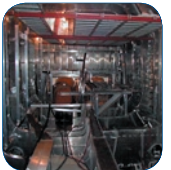
The M/V CHENEGA will be delivered in 2005 and is the second fast ferry built by Derektor for the AMHS. This photo is of the starboard engine room looking aft at the generator foundation and electrical panel tube supports getting installed.
