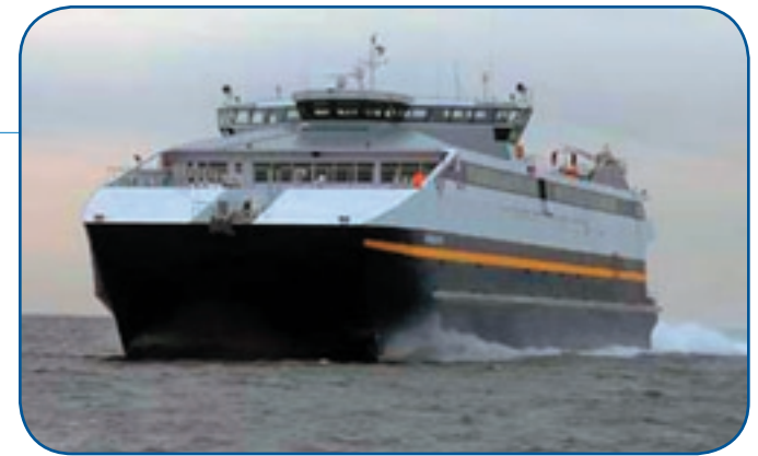
The new fast ferry FAIRWEATHER went into service earlier this year. The vessel is powered by four diesel engines and four water jets.
