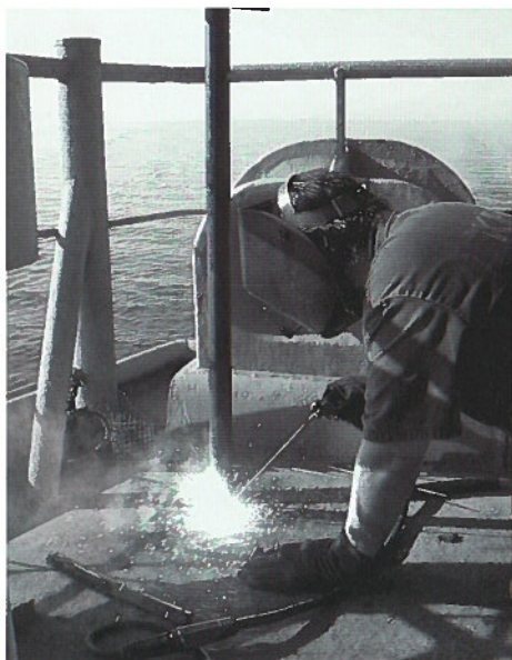
1st A/E Dave Andersen welding a machine gun mount on deck of the CAPE RAY for force protection while sailing in support of OIF.
