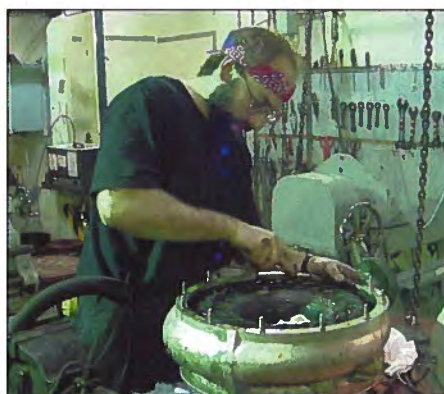
2nd A/E Ron Petrocelli, performing an overhaul of the compressor side of the GREENPOINT's Diesel Generator Turbocharger unit.
