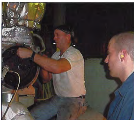
Aboard the GREENPOINT are 1st A/E Mike Buckley III (l) and 3rd A/E Steve Curley (r) who are overhauling the Auxiliary Diesel Generator Turbocharger unit.
