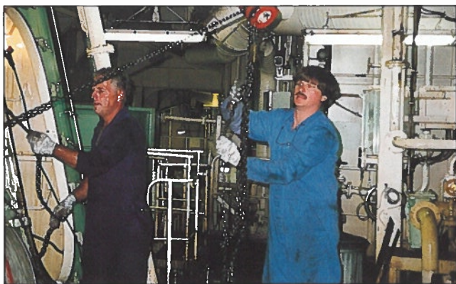
Aboard the C-11 vessel APL THAILAND are Steve Granahan and Karl Knudsen. The two are busy removing a main engine crankshaft bearing.
