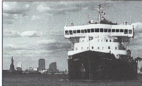
The Dredge ship MCFARLAND. The ship is the only one of its kind that has triple capability for direct pumpout, bottom discharge and sidescasting or boom discharge.
