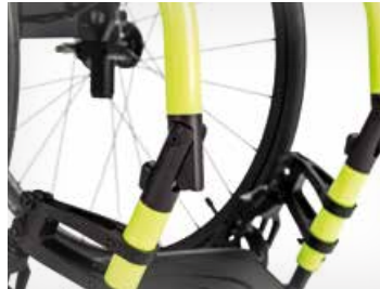
Optional front frame folding mechanism (+480gr).
